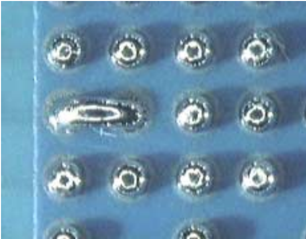
Fig. 7: Coalescence of stencil printed and reflowed eutectic balls caused by inhomogeneous amount of solder
