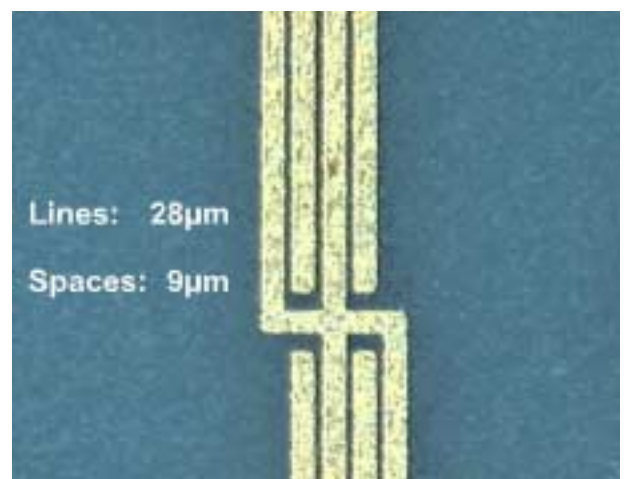
Fig.4: Example of the line resolution of Thin Film on an "as sintered" LTCC surface
