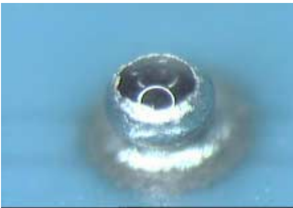
Fig. 12: Detailed picture of the damaged coating of the SOL balls; the polymer ball is transparent
