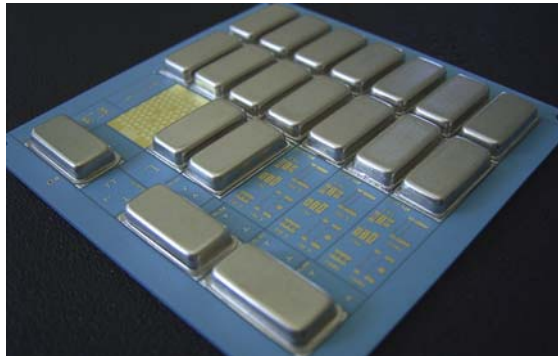
Fig. 3. Packaging of microwave BGA modules
